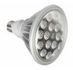
LED30W-PAR38-480V LED PAR38FLamp Type: LEDFWatts: 255Lumens: 2500DDimensions: 4.79" (121.65mm) OD 4.74" (120.32mm) Total Height- 3.61" (91.64mm)3Voltage: 347-480 VAC 50/60Hz - 3 Phase or Phase to PhaseIfColor: White (Red, Green, Blue, Amber, and Infrared also available. There may be longer<br/>lead times on specialty colors)RCRI: >84 (White)S
