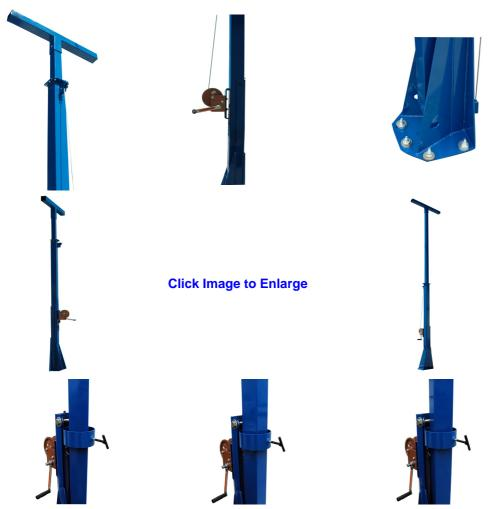
The LM series of towers are powder coated with glossy blue finish for corrosion resistances and aesthetics. These light masts are typically mounted to trailers or other stable surfaces via a 18" by 18" by 3/8" thick mounting base-plate which has been drilled to accept six 9/16" anchor bolts. A 44" wide and 3" by 3" by 1/4" thick mounting plate is attached to the upper section of the mast which provides a strong and stable platform for light fixtures and equipment.
