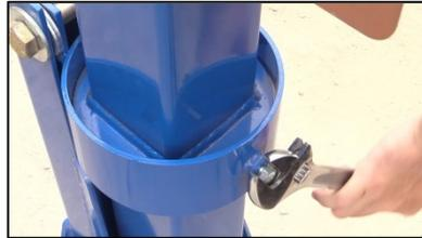
**DO NOT ROTATE MAST MORE THAN 90°** to prevent tangling cord around light mast. *Ensure cables are not in the way or tangled when lowering mast!*
