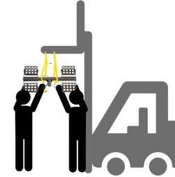
7. A ladder will need to be placed on both sides of the mast, in order for 2 people to guide the head in to place.
