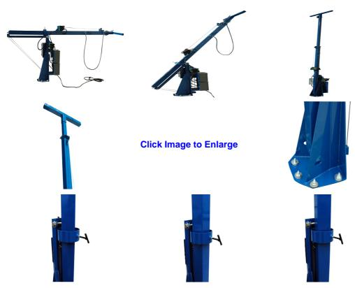
The LM series of towers are powder coated with glossy blue finish for corrosion resistances and aesthetics. These light masts are typically mounted to trailers or other stable surfaces via a 15" by 13" by 1/4" thick mounting base-plate which has been drilled to accept six 9/16" anchor bolts. A 44" wide and 2" by 2" by 1/4" thick mounting plate is attached to the upper section of the mast which provides a strong and stable platform for the mounted fixtures or equipment.
