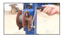
**WARNING:** Power cables can become pinched or tangled around light mast while lowering or rotating. Take caution in keeping cables clear.
