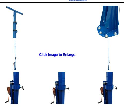
The LM series of towers are powder coated with glossy blue finish for corrosion resistances and aesthetics. These light masts are typically mounted to trailers or other stable surfaces via a 15" by 13" by 1/4" thick mounting base-plate which has been drilled to accept six 9/16" anchor bolts. A 44" wide and 2" by 2" by 1/4" thick mounting plate is attached to the upper section of the mast which provides a strong and stable platform for light fixtures and equipment.
