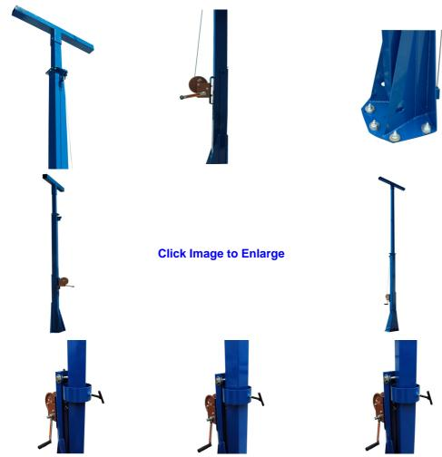
The LM series of towers are powder coated with glossy blue finish for corrosion resistances and aesthetics. These light masts are typically mounted to trailers or other stable surfaces via a 24" by 24" by 3/8" thick mounting base-plate which has been drilled to accept six 9/16" anchor bolts. A 44" wide mounting plate is attached to the upper section of the mast which provides a strong and stable platform for light fixtures and equipment.
