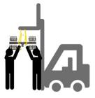
**7.** A ladder will need to be placed on both sides of the mast, in order for 2 people to guide the head in to place.
