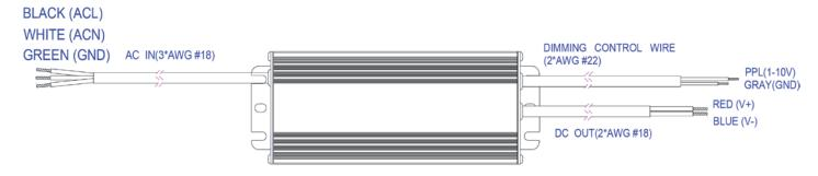
Output Current - 4000 mA Input Voltage Range - 90-305V AC Output Voltage Range - 12-24V DC Maximum Output - 96 Watts Typical Efficiency - 87%
