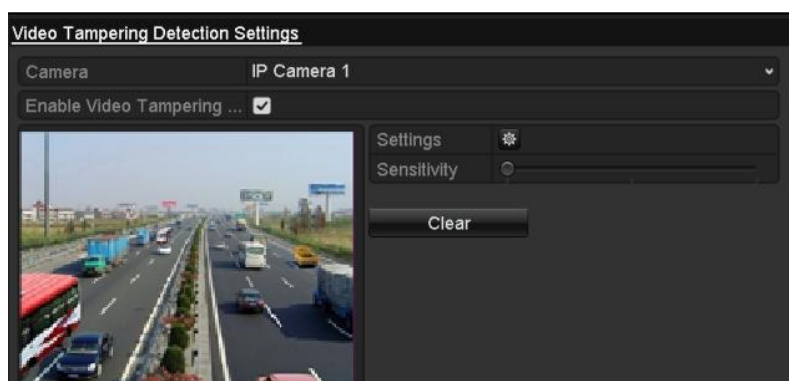
Figure 8. 11 Video Tampering Setting Interface
