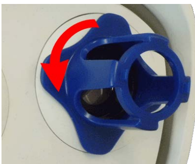
Fig. 52: Turn sensor module counter-clockwise until it stops
