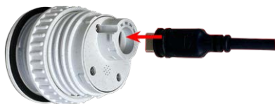
Fig. 11: Connect the sensor module cable
