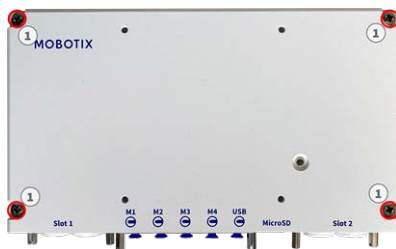
Fig. 37: Mounting plate installed on wall
