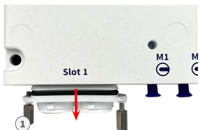
Fig. 32: Remove cover from interface board slot
