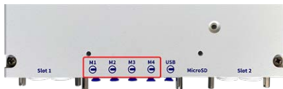
Fig. 39: Module connectors of the MOBOTIX S74
