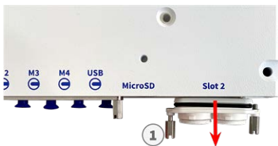
Fig. 22: Remove cover from interface board slot
