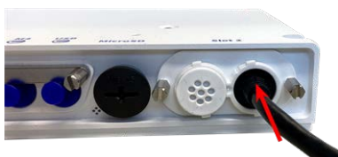
Fig. 41: Press the plug in firmly until the blue sealing ring clicks into place
