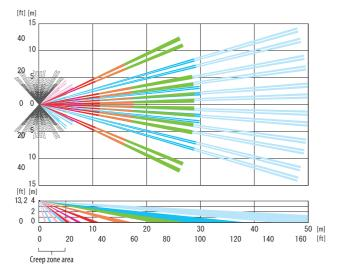
Detection angle of the creep zone can be adjusted  $\pm 135^\circ$  horizontally as shown in gray.
