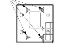
6) Hang the wall switch onto the socket cap screws and tighten down with the allen wrenches provided in the parts bag or with the handle grip allen wrenches. Alternate the tightening of the screws a few turns at a time each from the top to bottom.
