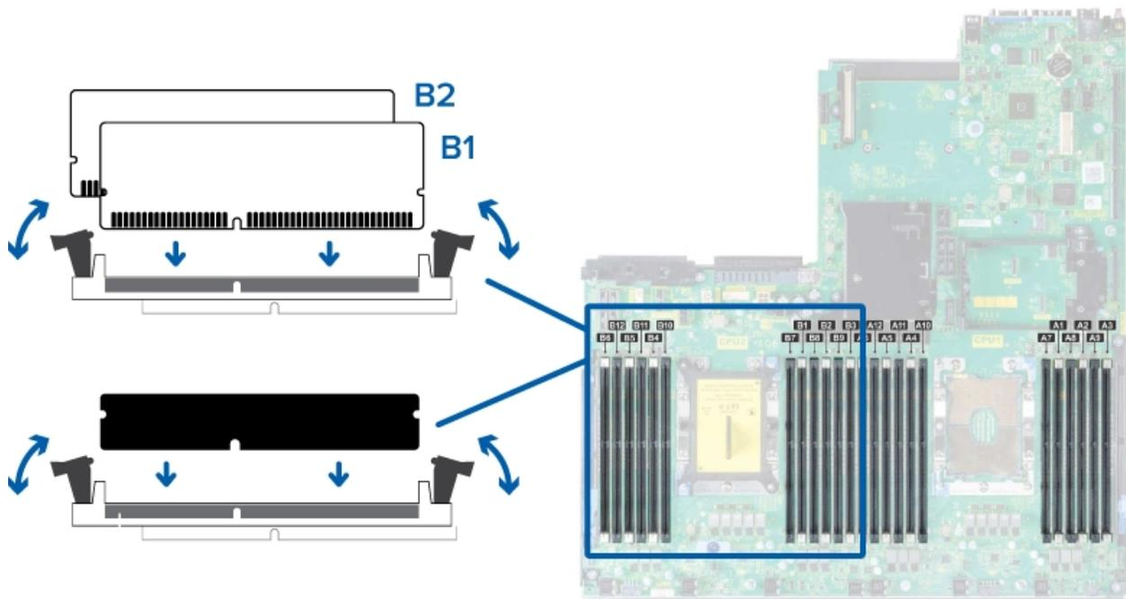
**Important:** To prevent damage to the memory module or memory module socket during installation, do not bend or flex the memory module. You must insert both ends of the memory module simultaneously.
