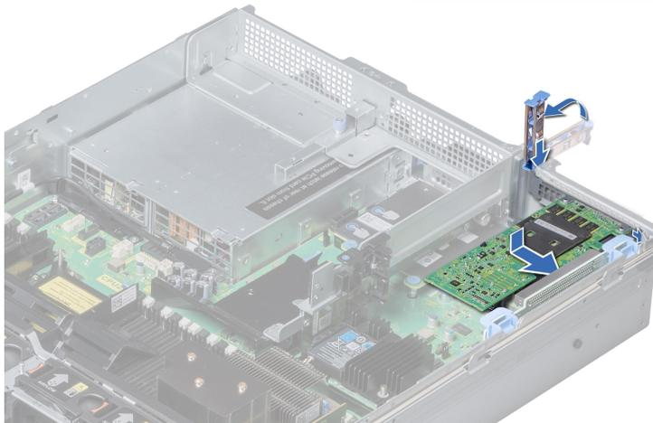
6. Align the connector on the GPU card with the connector on the riser.
