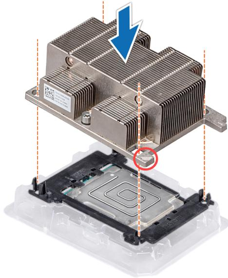
7. Align the pin 1 indicator on the heat sink to the system board and then place the processor and heat sink module on the processor socket.
