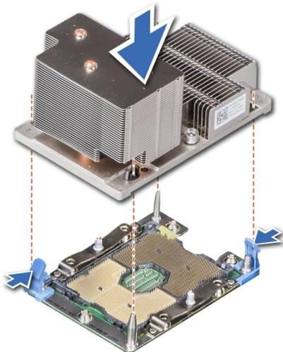
**Important:** Do not force the processor into the socket. The processor should slide easily into the socket when aligned correctly.
