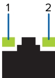
Figure 2: (1) Link LED. (2) Connection Status LED.
