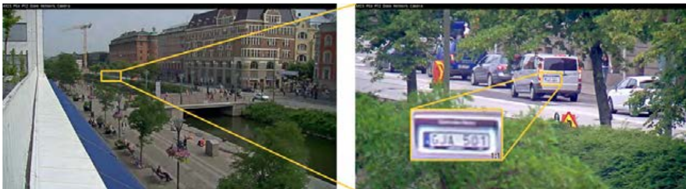
Images from AXIS P54. Left: wide view. Right: 18x zoomed-in view where the license plate of a vehicle 200 m (660 ft) away can be read.
