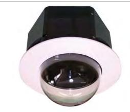
The 7" indoor recessed dome housing is ideal for indoor use where a plenum rated enclosure is required. This dome has a steel body and trim ring, and a polycarbonate clear or tinted capsule. Its larger size allows for additional electronic devices to mounted within the dome. Its high quality capsule is also ideal for indoor mounting of high zoom PTZ cameras.
