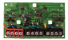
The ICP-SDI-9114 SDI Splitter allows the set up of two independent, isolated SDI buses from a single SDI connection on the control panel. When this accessory is installed with a control panel and wired to create separate SDI buses for fire and intrusion devices, the system is a UL864 compliant combination control panel.
