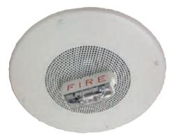
The Wheelock S8-24MCC-FW Multi-candela Speaker Strobe provides high audible output with clear audibility at either of its field-selectable voltages (25 VRMS or 70 VRMS) and at all of its field-selectable powers (1/8 W, 1/4 W, 1/2 W, 1 W, 2 W, 4 W, or 8 W). With its multi-candela (15 cd, 30 cd, 75 cd, or 95 cd) strobe it meets the needs of the life safety industry for effective emergency voice communications, tone signaling, and visible signaling to alert the hearing impaired.
