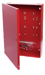
The AE4 is a large red enclosure that accommodates an optional tamper switch for monitoring the door. It is made of 1.2 mm cold-rolled steel and includes a keyed lock. It measures 52.7 cm x 38.1 cm x 10.8 cm(20.7 in. x 15 in. x 4.25 in.).
