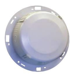
A circular metal back box for use with 8-inch ceiling-mount speakers. It has an overall (flange) diameter of 31.3 cm (12.3125 in.), an interior diameter of 24.8 cm (9.75 in.), and a depth of 10.3 cm (4.1 in.).
