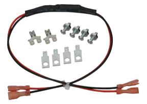
The D122 Dual battery harness protects the installer and battery when connecting two batteries, in parallel, to compatible control panels. The D122 eliminates the hazards of batteries connected in parallel by utilizing a thermal circuit breaker to govern the circuit. It breaks the electrical circuit of the second battery when the thermal rating is exceeded.
