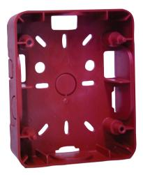
The GSB Surface Back Box is constructed of durable plastic and measures 5.6 in. x 4.6 in. x 1.5 in. (14.1 cm x 11.6 cm x 3.7 cm). It has half-inch conduit knockouts with metal washer reinforcement.
