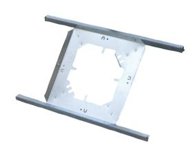
The SSB-8 Ceiling Support Bridge is a steel support bridge for mounting notification appliance in areas with suspended ceilings. It measures 23.75 in. (60.3 cm) long by 14.5 in. (36.8 cm) wide.
