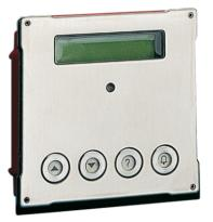
Module made using double 2.5 mm 316 stainless steel plate, complete with 4 backlit buttons and 32-digit alphanumeric display. Stores up to 1000 user names. Scroll through names using 2 search buttons. Once the name is displayed, simply press the call button. Dimensions: 106x106x56 mm. Compatible only with the art. 4680, 4680C, 4681, 4682HC, 1621, 1621VC, 1622, 1622VC, 1682 and 1682HVC combined with the fronts art. 3262S/x and 3268S/x.
