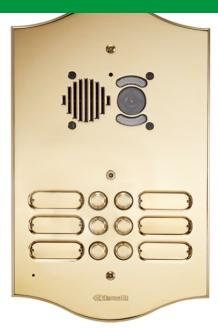
Video entry phone entrance panel with front plate in 3 mm thick watchmaking brass plate with PVD treatment. Complete with flush-mounted box and anti-intrusion screws. All entrance panels are fitted with bulb sockets (without bulb) for festoon bulbs with a diameter of 6.3 x 39. The keypad should be finished with an audio/video unit depending on the wiring system used. 3 buttons, 1 wire. Plate dimensions 135x293x3 mm. Box dimensions 115x227x55 mm. 1 bulb socket
