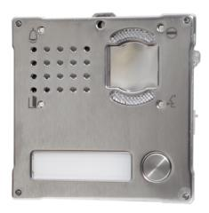
Module made using double 2.5 mm 316 stainless steel plate. For use with audio/video unit depending on the wiring system used. 1-button module. Dimensions 106x106x44 mm
