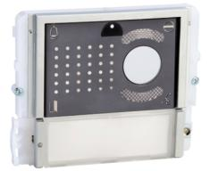
Module designed for audio/video speaker unit, with stainless steel finish faceplate. Nameplates with LED lighting (options: blue, white or off). To be fitted with a suitable door entry speaker unit depending on the cabling system used. Dimensions 112x89.5x32 mm.
