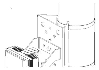
A single illuminator can be mounted to the bracket using M6 nuts and bolts. Vertical adjustment can be made using the two hex bolts on each side of the illuminator. Mounting holes are also provided to pair with single (DW-ILWM1), double (DW-ILWM2) and triple mounting (DW-ILWM3) brackets.
