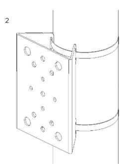
Place the bracket against the pole in the required position. Thread the steel straps through the slots located in the bracket and tighten around the pole with a suitable wrench.
