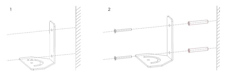
Use the bracket to mark and drill the necessary holes in the wall.
