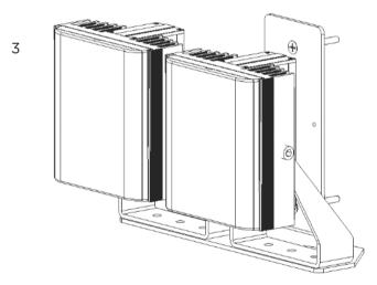
With the bracket secured to the wall, attach the illuminators with the supplied M6 nuts and bolts. For each illuminator, attach the center bolt first then rotate the illuminators to the required horizontal position. Once the necessary position is achieved, secure the illuminators with the remaining nut and bolt in one of the outer holes.
