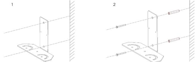
Use the bracket to mark and drill the necessary holes in the wall.
