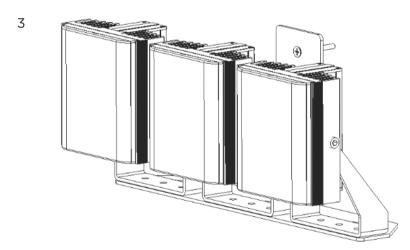
With the bracket secured to the wall attach the illuminators with the supplied M6 nuts and bolts. For each illuminator attach the center bolt first then rotate the illuminators to the required horizontal position, then secure with the remaining nut and bold in one of the outer holes.
