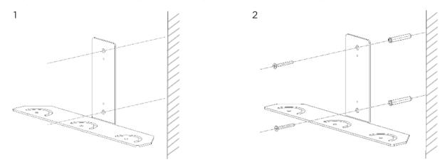
Use the bracket as a template to mark and drill the necessary holes in the wall.
