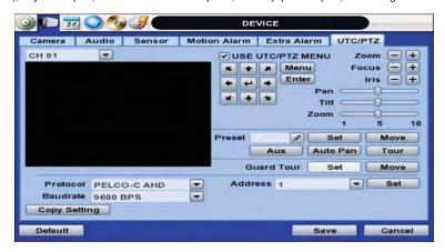
Adding a PTZ camera: Once a PTZ camera is properly connected to the DVR using the RS485 ports, go to the PTZ setup menu and adjust the following values:
