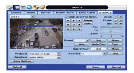
UTC is remotely set to camera OSD menu in the DVR. Select the proper protocol of the connected camera. Non-check the 'USE PTZ MENU' mode, set the menu and adjust as below.
