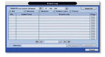
**NOTE** If an alarm or event does not appear in the event log, check the alarm settings, and connection port at the DVR's back panel..
