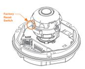
Resetting the camera: To reset the camera, use the tip of a paper clip or a pencil and press the reset button. Pressing the button for five (5) seconds will initiate a camera-wide reset of all the settings, including network settings.
