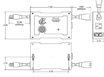
Visual, audible, smart. **DITEK's DTK-LC2** sets a new standard for 120V AC power filtering with surge protection. Its design provides maximum critical load protection by minimizing AC supply voltage spikes and isolating incoming surges that originate from lightning or other sources. The DTK-LC2 features an LED health status indicator that extinguishes and sounds an audible alarm when protection has been compromised. This device can be wall mounted or placed on a table top.
