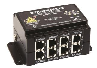
**DITEK's DTK-WM4EXTS** is a 4-channel, wall mount surge protector that uses state-of-the-art circuitry to provide best-in-breed surge protection for shielded PoE extender circuits. It supports data speeds up to 10GbE, and provides surge protection grounding to remote devices when used with STP cabling. The DTK-WM4EXTS is ideal for smaller installations where Ethernet cabling feeds require protection before entering PoE extender devices.
