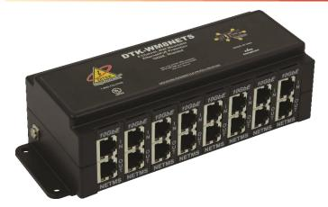
**DITEK's DTK-WM8NETS** is an 8-channel, wall mount surge protector that uses state-of-the-art circuitry to provide best-in-breed surge protection for shielded Ethernet, PoE and optional PoE extender circuits. It supports data speeds up to 10GbE, and provides surge protection grounding to remote devices when used with STP cabling. The DTK-WM8NETS is ideal for smaller installations where Ethernet cabling feeds require protection before entering network switches.
