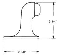
*No. 3340X*—Heavy duty cast brass or cast bronze. Conforms to ANSI/BHMA 156.16. Brass/Bronze L12131 conforms to Fed. Spec. No. 1328 E. Bumper contact height 2 1/4".
