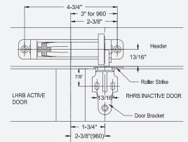
When the active and inactive doors are open, the coordinator arm pivots downward, positioning the arm and rubber roller below the top of the active door. As the active door is closed it comes in contact with the arm and roller and is held open. When the inactive door is closed, the nylon roller on the coordinator mechanism comes in contact with the roller strike and lifts the projecting arm above the top of the active door, allowing it to close in sequence.
