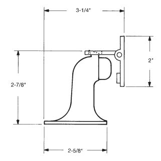
*No. 3347X*—Heavy duty cast brass or cast bronze. Floor stop with cast strike and hinged holder. Hinged holder engages cast projection on top of floor stop. Raising the holder releases the door. Conforms to ANSI/BHMA 156.16. Brass/Bronze L11371 conforms to Fed. Spec. No. 1329 E. Bumper contact height: 2 1/4".
