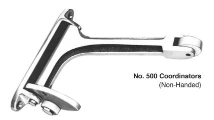
No. 500 Series Coordinators are nonhanded, UL listed devices used to coordinate the closing of pairs of doors in jamb openings 36" to 104" wide. Coordinator mechanism and inactive door brackets are cast of solid brass or bronze. The roller strike for top of inactive door is wrought stainless steel, brass, or bronze.
