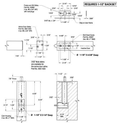
*Door Preparation:* To prep the door for the 960 Bolt, only two 1-1/8" diameter holes are required. The top bolt is installed first, and then the edge bolt. The edge bolt's grooved channel will engage the top bolt's grooved bottom, locking them together.
