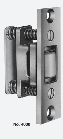
Adjustable roller latches are a versatile piece of hardware which can be used for a variety of applications. Roller latch easily adjusts to provide the desired contact between roller and applicable frame strike. Latch pressure is adjusted without removing the roller latch from the door.
