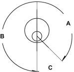
**C. Battery Service** - Turn key counterclockwise pass "OFF" position. The alarm module, extruded cover, and end cap slides out of the housing as one complete unit to expose the battery.
