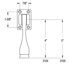
*No. 3104-4" & 3105-5"*—Rugged cast iron kick down holders conform to ANSI/BHMA 156.16. Hinged arm held up by spring locks. Serrated rubber shoe holds door firmly in any position. Rubber shoe is threaded for easy, secure replacement
