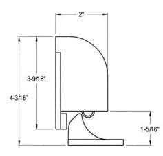
*No. 3467X*—Conforms to ANSI/BHMA 156.16, L11301. Easy operation with a push and pull on the door for open and release. Durable die cast brass construction for heavy traffic areas. The holder is mounted on the door, and the strike on the floor. Designed to accommodate a wide range of door to floor clearances. Supplied with a universal screw package for all types of applications.
