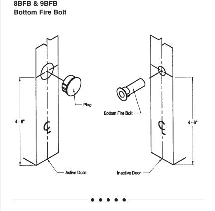
The 805, 840, 905, 940, and 960 Automatic and Self Latching Top Flush Bolts are UL Listed for pairs of fire doors when specified with the 8BFB or 9BFB Bottom Fire Bolt.
