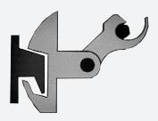
**PANNEX PATENTED INTERLOCK** Strike and latch are investment cast stainless steel heat treated and tempered to Rockwell C 43, approx. tensile strength 200,000 P.S.I.
