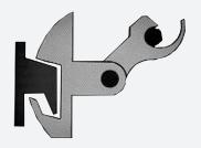
**PANNEX PATENTED INTERLOCK** Strike and latch are investment cast stainless steel heat treated and tempered to Rockwell C 43, approx. tensile strength 200,000 P.S.I.
