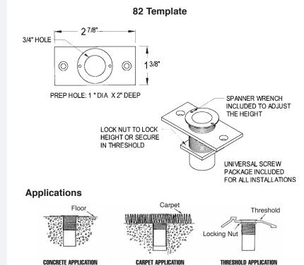
The 82 Universal Dust Proof Strike is designed to eliminate dust and debris from collecting in the floor strike. The plate is both adjustable and removable, making it versatile for carpet, threshold, or concrete applications. It is compatible with all types of DCI flush bolts.
