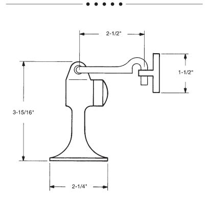
*No. 3367X*—Heavy duty cast brass or cast bronze. Floor stop with cast hook and holder. Conforms to ANSI/BHMA 156.16. Brass/Bronze L11371 conforms to Fed. Spec. No. 1329 E. Bumper contact height: 2 5/8".
