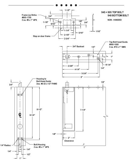
Up to 8' x 9' Wood Door Pairs 1-1/2 Hour Fire Rating
