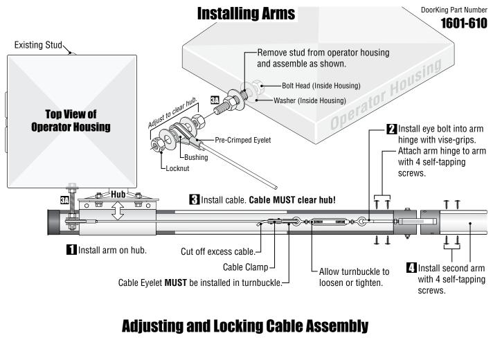
After adjusting cable tension, lock turnbuckle with nuts to keep turnbuckle from twisting.
