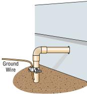
**IMPORTANT:** Ground wire shown without safety protection for clarity. Make sure ground wire is protected from being touched or electrical shock could occur!
