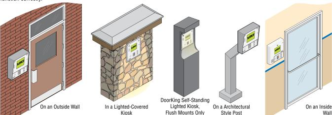
WARNING If this telephone entry system is used to control a vehicular gate with an automatic gate operator, the telephone entry system must be mounted a minimum of six (6) feet away from the gate and gate operator, or in such a way that the user cannot come into contact with the gate or gate operator when using this entry system.
