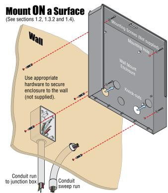
Examples of conduit runs that may be used, depending on how you choose to run the wiring. Some installations will allow the conduit to be run outside the wall and connect to the bottom of the enclosure but this is generally NOT recommended.
