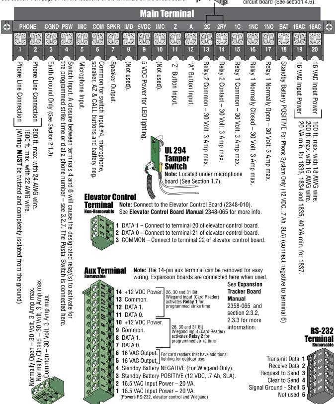
**Note:** Located in the upper left corner of circuit board. The 6-pin terminal can be removed for easy wiring. Connects a PC (See Section 2.5.1).
