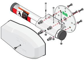
**Lighted Arm Note:** Unplug wire harness and remove from operator housing **BEFORE** unbolting arm from hub.
