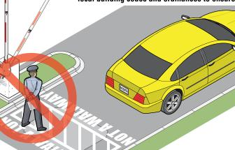
**IMPORTANT:** A barrier gate operator installed **WITHOUT** any safety sensors **CANNOT** sense a person under the raised arm and can strike them while the arm is lowering.
