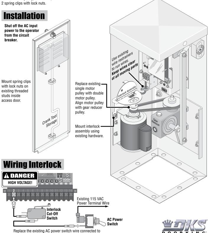
terminal #2 with interlock cut-off switch wires.
