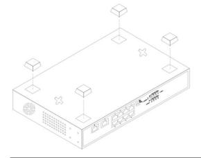
**Note:** Make sure to leave at least 10 cm of space around the switch for adequate ventilation.
