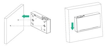
**Note:** Make sure to leave at least 10 cm of space around the switch for adequate ventilation.
