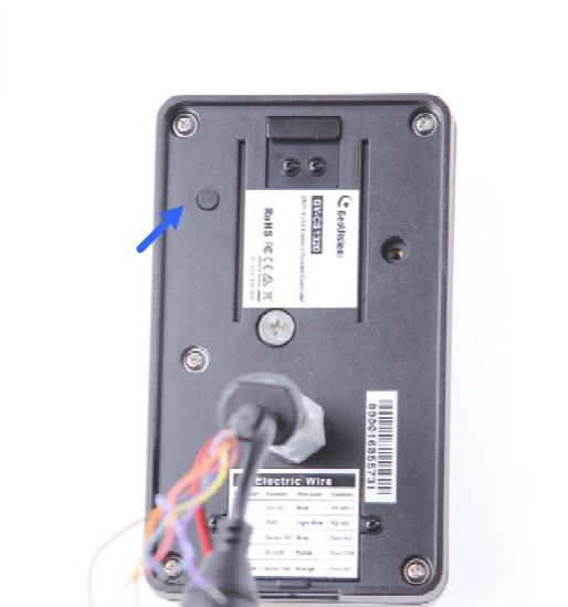
3. Wait until the status LED blinks twice to release the **Load default** button. The process takes about 5 seconds.
