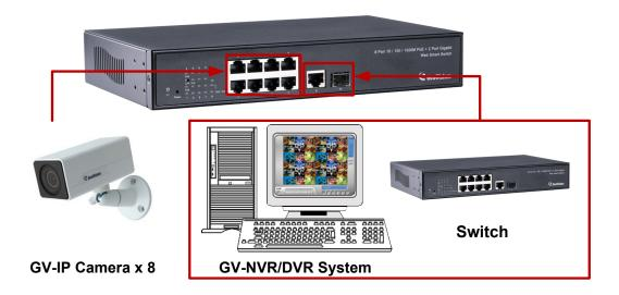
**Note:** The maximum cable length for Gigabit RJ-45 is 100 meters. For connection that exceeds 100 meters, you can use the Gigabit SFP ports.
