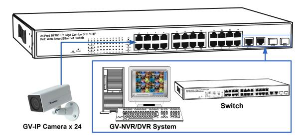
**Note:** The maximum cable length for Ethernet is 100 meters. For connection that exceeds 100 meters, you can use the Gigabit SFP ports.
