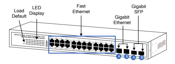
**Important:** For the usage of Gigabit Ethernet and Gigabit SFP ports, you can only choose one port from group A and one port from group B to connect. Both groups offer one of their ports for connections at a time.
