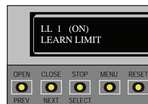
Figure 42. Resetting OPEN and CLOSE Limits
