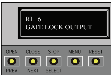
Figure 62. Setting the User Relay Function in the Installer Menu
