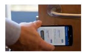
solution, users are no longer required to carry a card to access doors within a facility. They can now use their mobile phone instead. With a simple tap of the screen, users can gain quick and efficient access to any door with a HID BLE door reader. Credentials can be easily created/edited through the EntraPass system. An email invitation can be sent to a user and mobile IDs issued.
