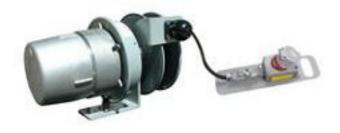
EPLRT-25-12.3-HR Explosion Proof Cord Reel w/ Tool Tap Standard Features: 25` 12/3 SOOW cable Spring activated ratchet 4-roller adjustable cable guide and ball Built to UL 508 table 36.1/NEC Standards Indoor or Outdoor Use Rugged fabricated steel and cast aluminum slip ring enclosure Gray epoxy finish on all steel parts 6` feeder cord on fixed end 5-20 (125V) or 6-20 (250V) 20 Amp C1D1 outlet Dimensions: 24"W x 27.749"H x 26.35"D
