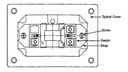
**CAUTION:** Use 12 AWG copper conductors only. Insert the bare wire conductor(s) under terminal clamp and securely tighten the screw(s). Note: Do not exceed 35 in-lbs. of torque.
